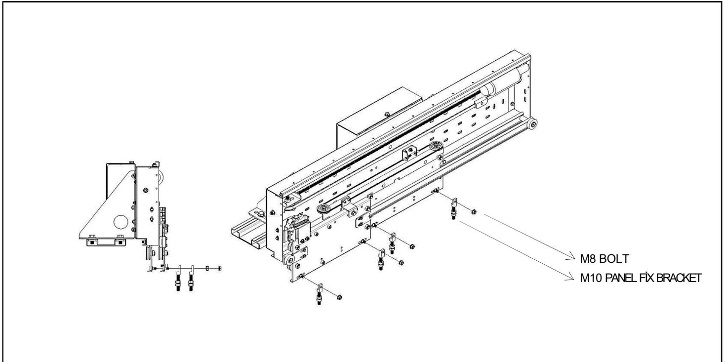
The panel hangers are attached to the panel carriages and fixed with M8 bolts.
