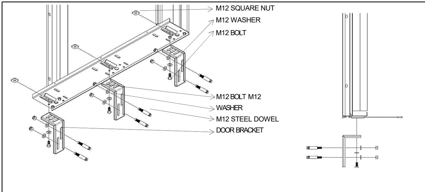
Floor door consoles are fixed to the wall with M12 steel dowels in the dimensions given in the technical details. Then the door frame and consoles are placed on it. Square nuts from the slots opened for M12 square nuts on the threshold are inserted into the slot and fixed to the door consoles.
