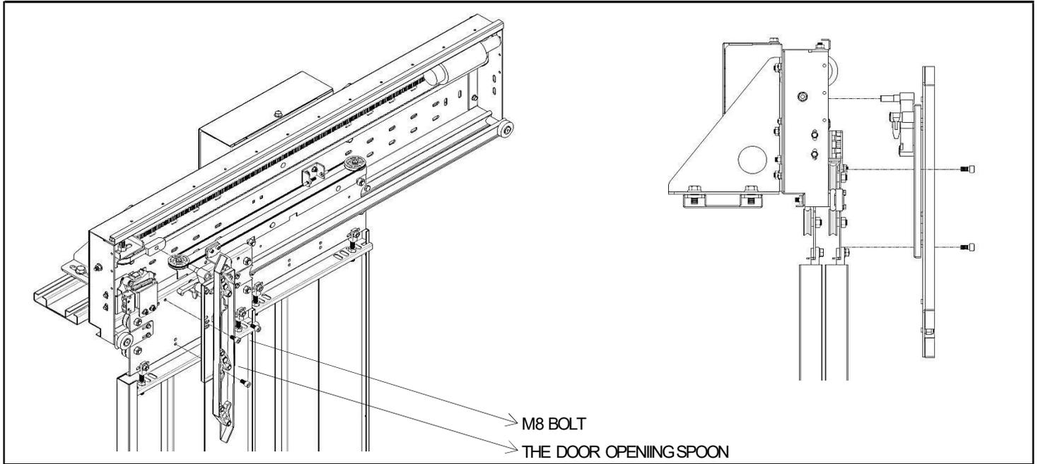
The door opening spoon is fixed on the panel trolley with M8 bolts.
