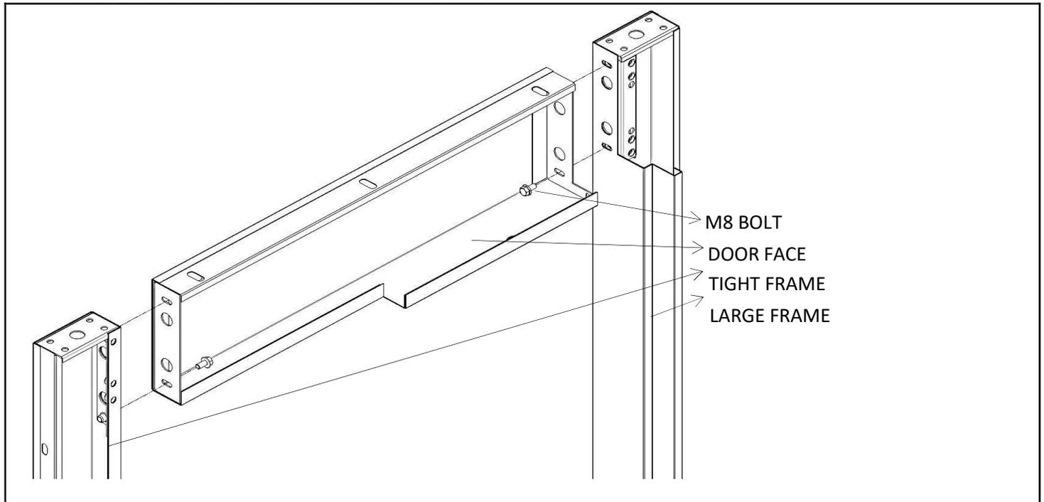
The narrow and wide frames of the door frame are fixed to the door forehead with 4 M8 bolts. It should be noted that the front side of the door frame is flush.
