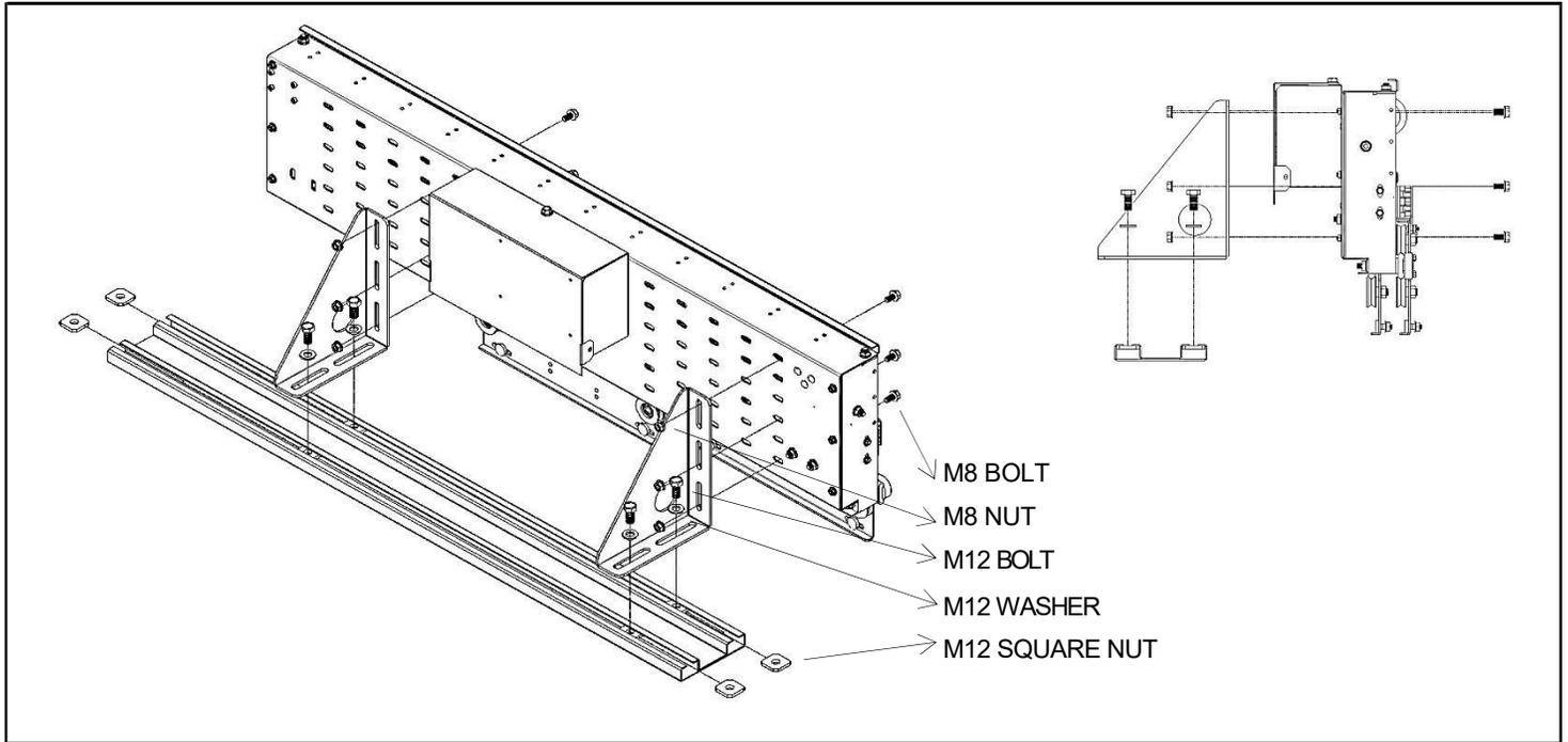
When installing the cabin door, first of all, the M12 square nuts are placed on the mechanism connection slides located on the cabin. The cabin door consoles are fixed on the cabin with M12 washers and bolts. The cabin door operator is fixed to these consoles.
