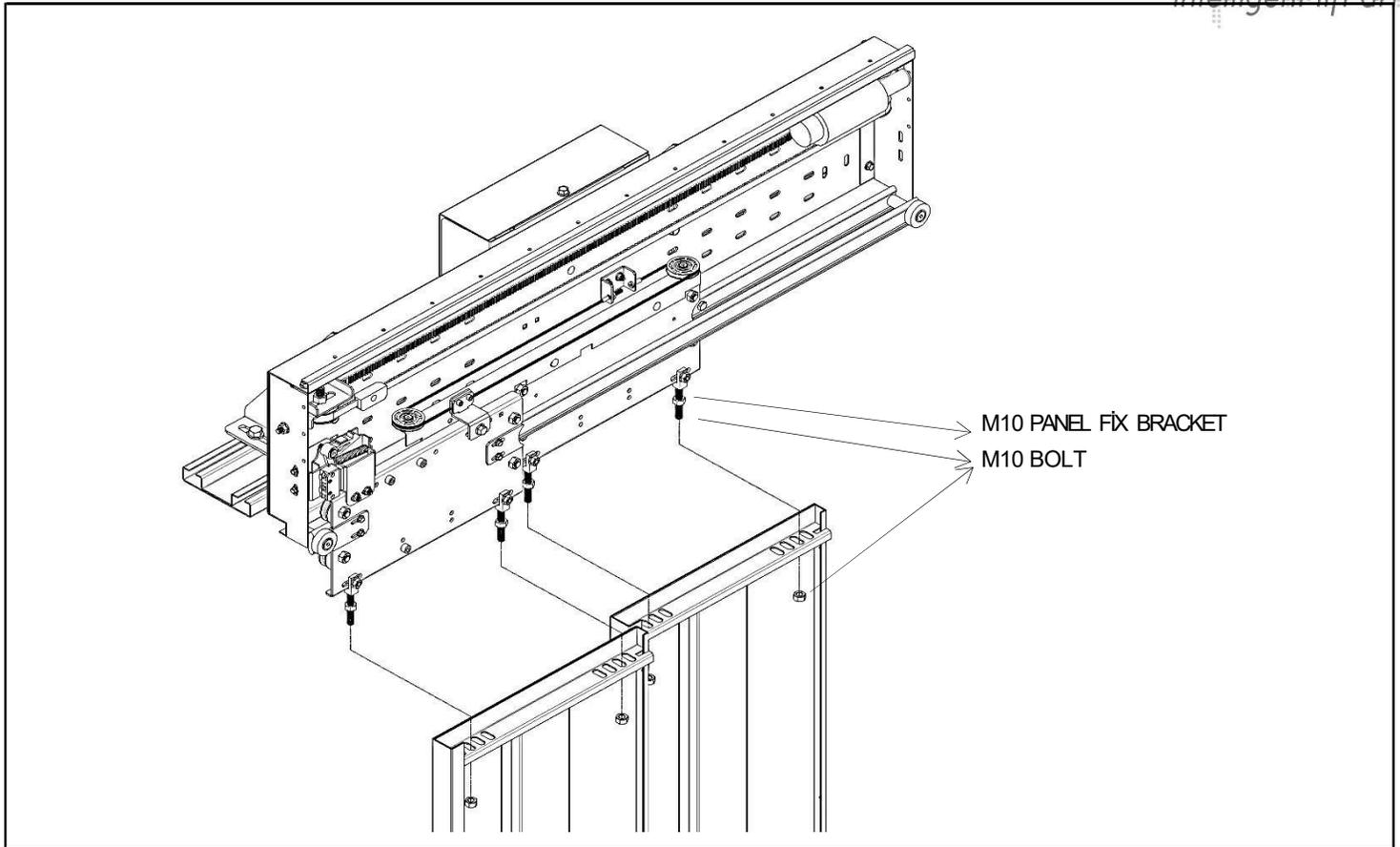
The panels are mounted on the panel car with the panel hangers in the dimensions given in the technical details. The panels can be adjusted in three axes.
