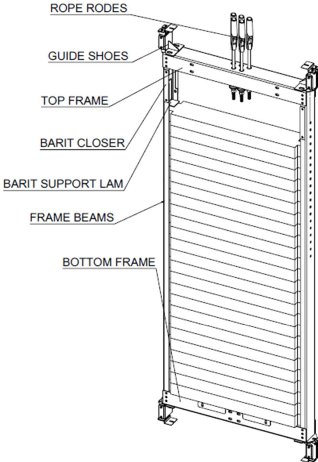
**10.1 Counterweight Weight Exploded Frame View**
