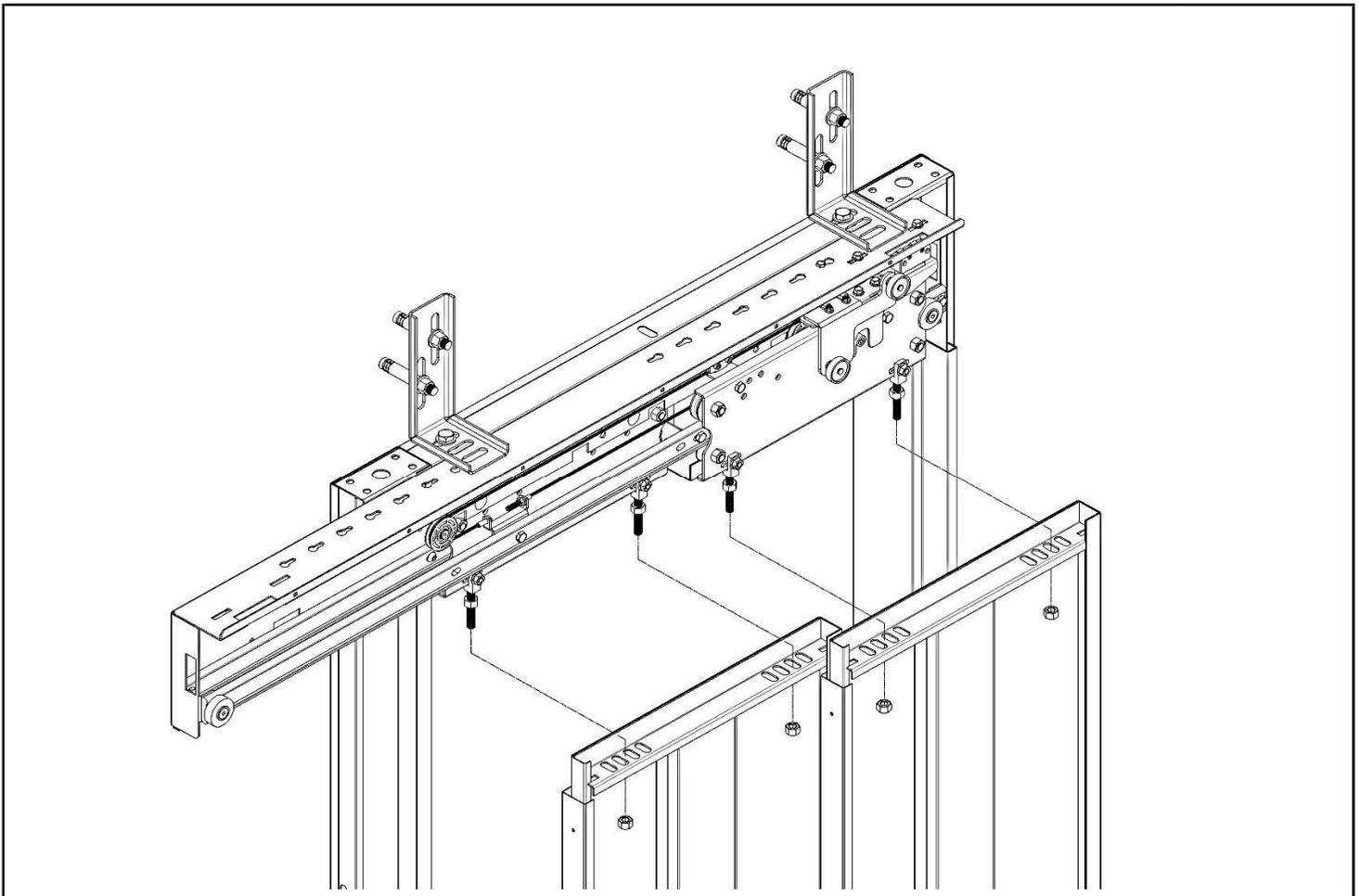
The panels are mounted on the panel car with the panel hangers in the dimensions given in the technical details. The panels can be adjusted in three axes.
