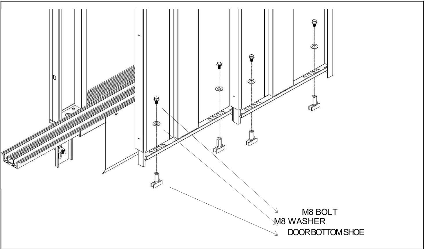
The door skates are first placed inside the aluminum threshold. Then M8 stamps from the slots located on the panel and it is fixed with bolts. Here, too, attention is paid to the fact that the door gaps are the same as the dimensions given in the technical details
