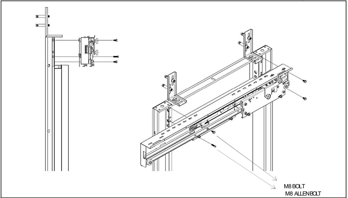
The floor mechanism is fixed to the door frame with M8 bolts as shown in the figure.
