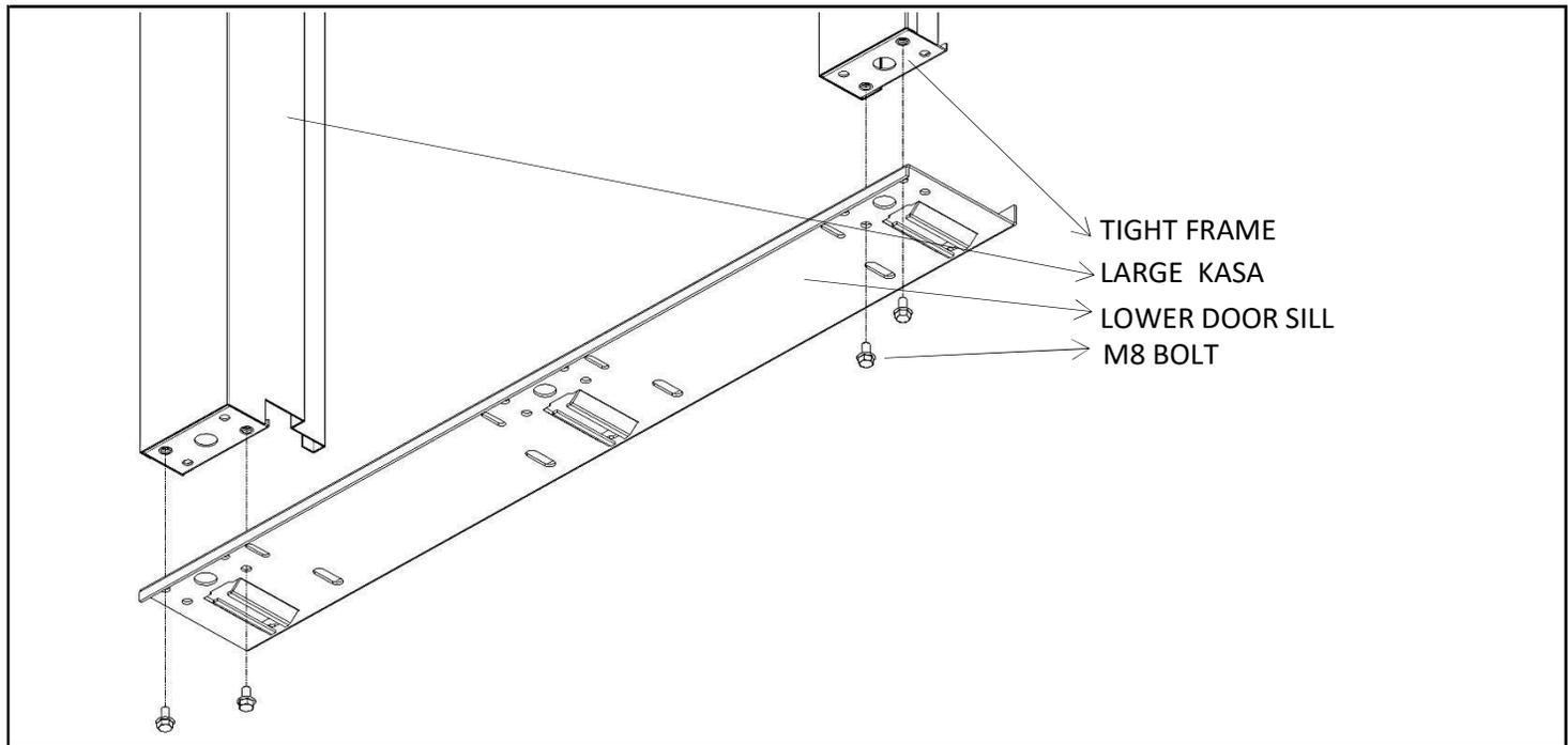
The narrow and wide frames of the door frame are fixed to the door bottom sill with 4 M8 bolts. It should be noted that the front face of the door frame is flush with the lower threshold of the door.
