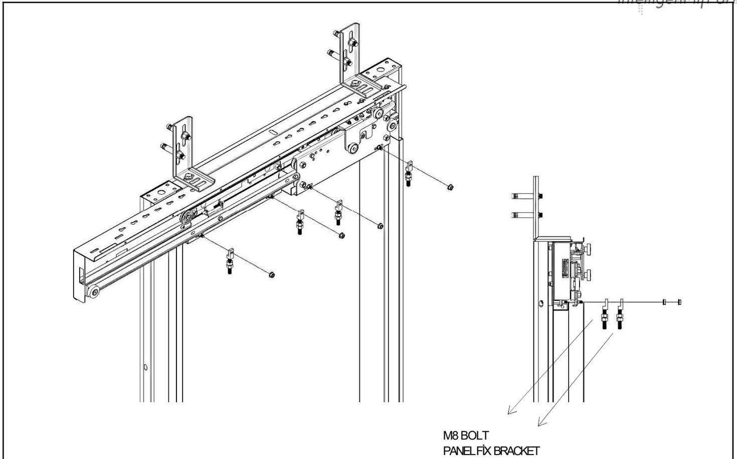
The panel hangers are attached to the panel carriages and fixed with M8 bolts.
