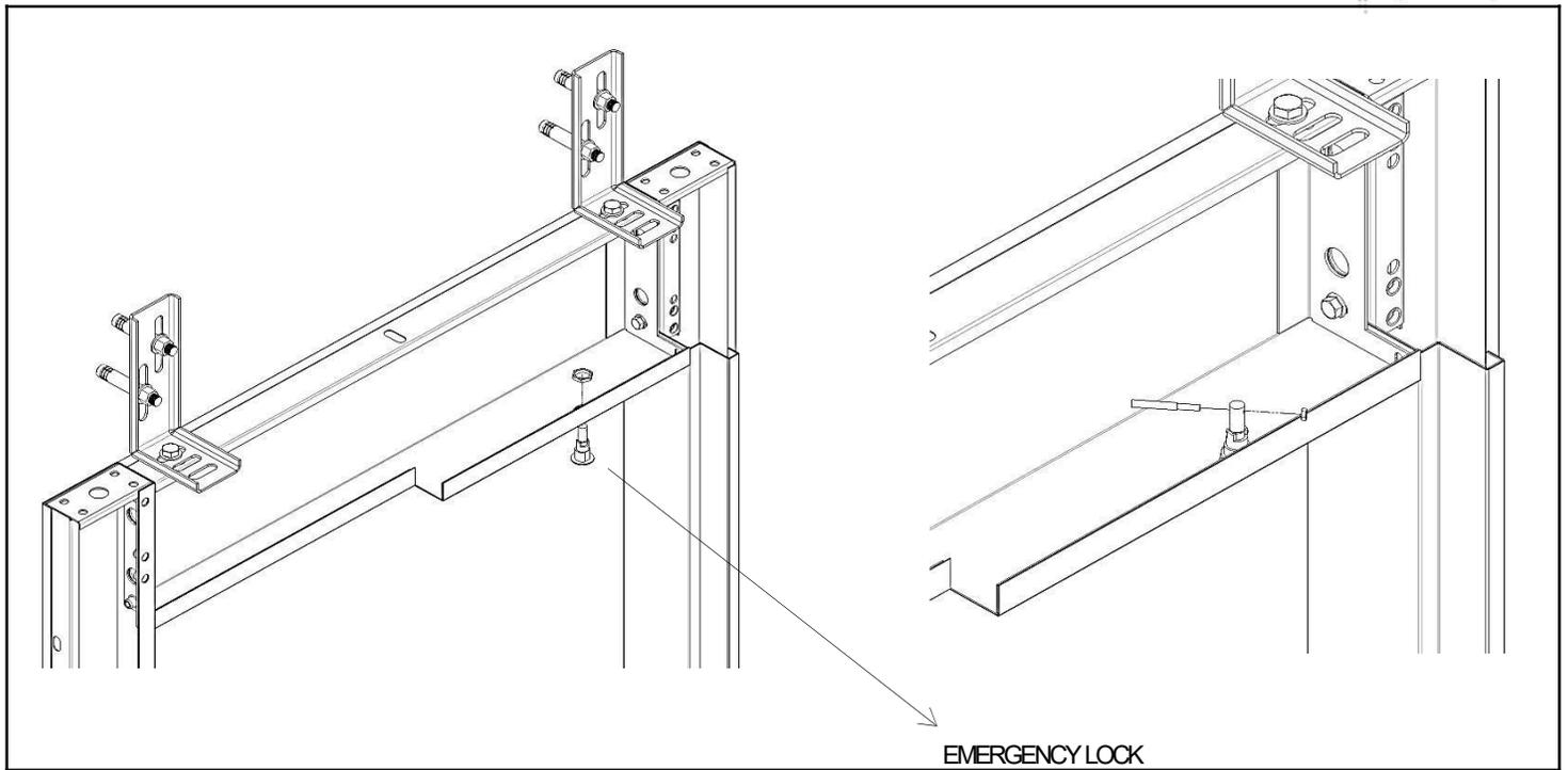
The emergency lock is attached to the slot located on the door forehead.
