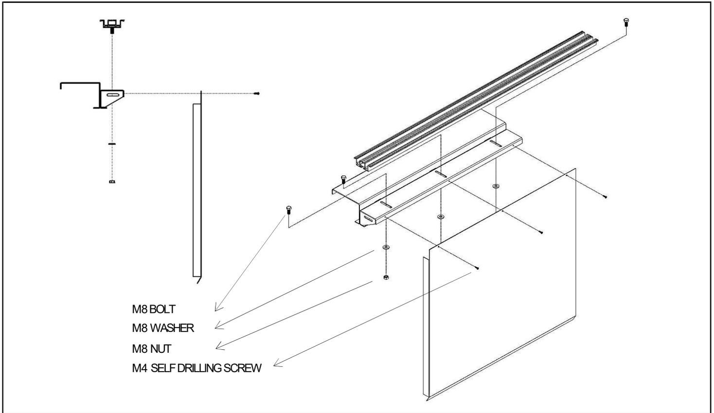
The aluminum threshold and the cabin skirt sheet are fixed to the door sill located on the cabin.
