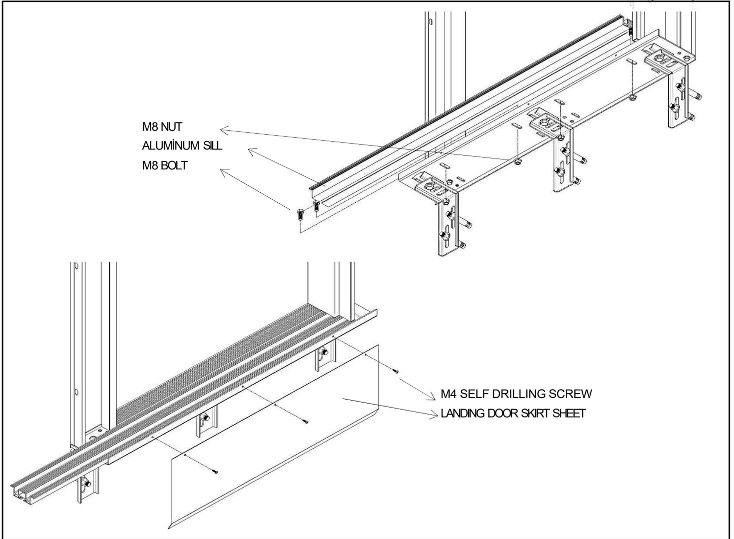
The aluminum threshold is fixed to the door bottom sill with M8 bolt.
