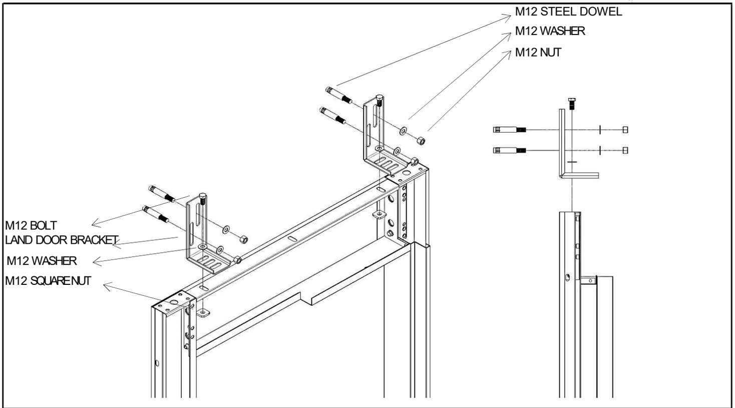
Floor door consoles are fixed to the wall with M12 steel dowels with the dimensions given in the technical details. Then the door frame is fixed to the wall with the M12 bolt from the slots located on the door forehead in a balanced way.
